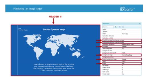
For Header 5 we define its height, its background image and its alignment. The background image includes a repeated design.
