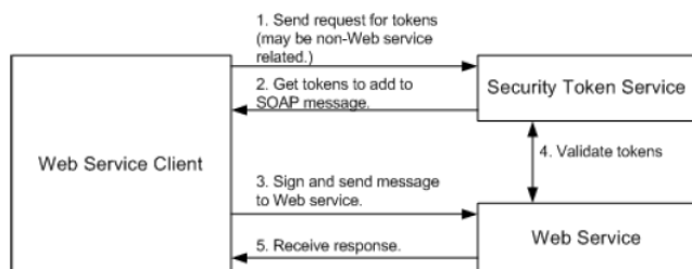
Typical Message Flow with WS-Security [WSS2]
