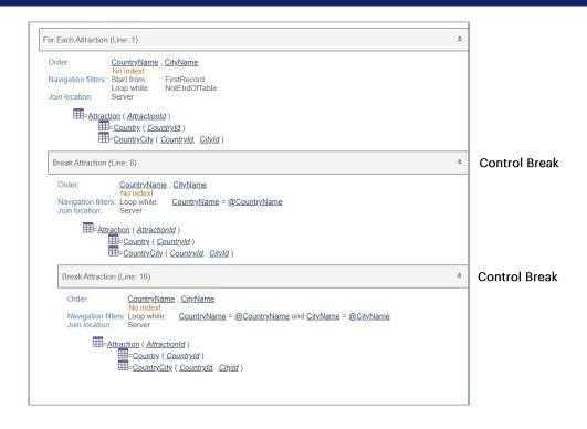
We have a double control break, which implies three For Each Commands If we look at the navigation list, we can see the word Break for every internal For Each, indicating the same base table, Attraction, and therefore, a control break.
