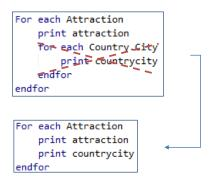
Note that here the second For Each command would be unnecessary, because for every attraction selected at a given moment in the external For Each command, there is only one related CountryCity record. So, this would be the same as not writing the second For Each command, and sending to print the CountryCity printblock that contains CountryName and CityName, which both belong to the Attraction extended table.
