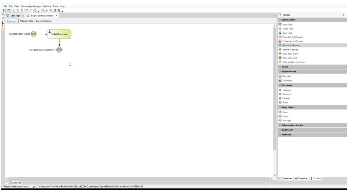
To represent a **decision** in the diagram we open the toolbox, drag an **Exclusive Gateway** node to the diagram and connect it from the TicketReservation task.
