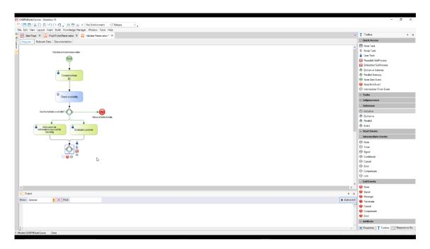
When paths are joined, an inclusive gateway synchronizes the paths through which the process actually moved. These are not necessarily all the paths to the gateway.
