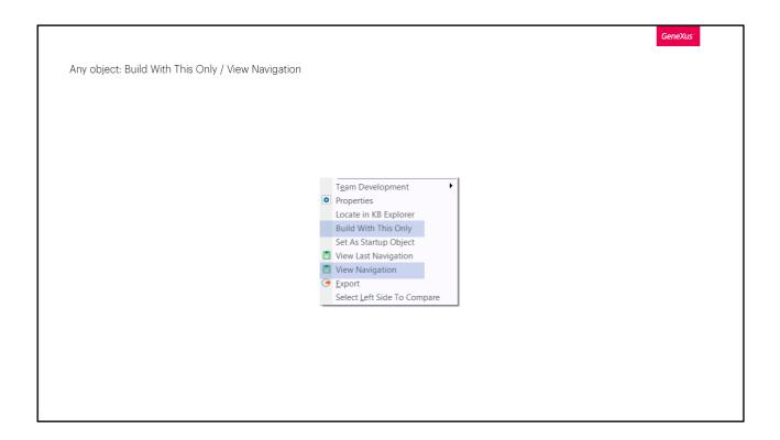
When we don't want the build process to be executed for the whole KB, but we want it to be done only for one object, we can right-click on it and select Build With This Only. If we are prototyping there, this will specify, generate, compile and eventually transfer to the cloud only the object we are interested in, whether it is a main object or not, and the result information will be in the Output window. If there is an error, the navigation list is opened to display it.
