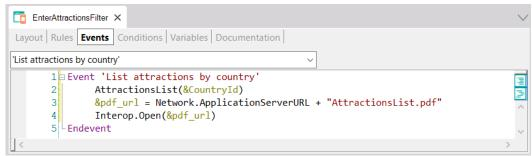
Set the panel as "Main program" and make sure that the AttractionsList proc has the value "Expose as web service" = True, "Rest Protocol" = True and "Call protocol" = Internal.
