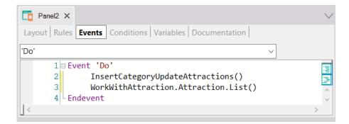
Again: the procedure with "Call Protocol" = Internal. Note that when invoking the procedure from the event, GeneXus automatically turns on the properties "Expose as Web Service" and "REST protocol" of the procedure. We take advantage of this and invoke the Work With List to see how the new attraction is listed.
